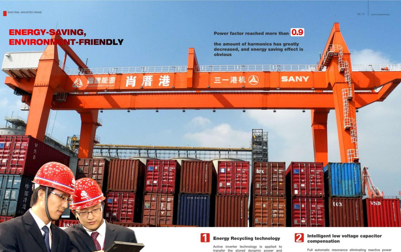
Active inverter technology is applied to transfer the stored dynamic power and potential power into electricity and be recycled to the grid. At the same time, it can resist the pollution to grid from higher harmonic voltage, thus increasing the power factor of the equipment.
